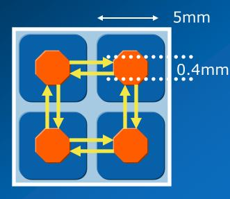
Packet Switched Mesh 16B=128 bit each direction 0.4mm @ 1.5u pitch 192GB/s Bisection BW
