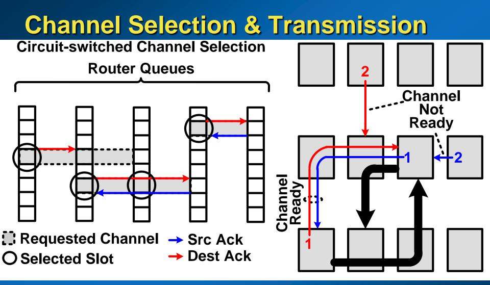
Queue slots store multiple channel requests Two acknowledges required to indicate ready channel More possible channels  $\Rightarrow$  87% throughput increase
