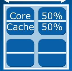
65nm, 4 Cores 1V, 3GHz 10mm die, 5mm each core Core Logic: 6MT, Cache: 44MT Total transistors: 200M
