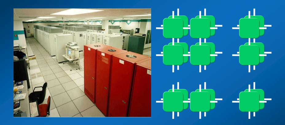
32 X 32 X 2 Mesh InterconnectSimultaneous bidirectional signaling50 GB/sec bisection bandwidth
