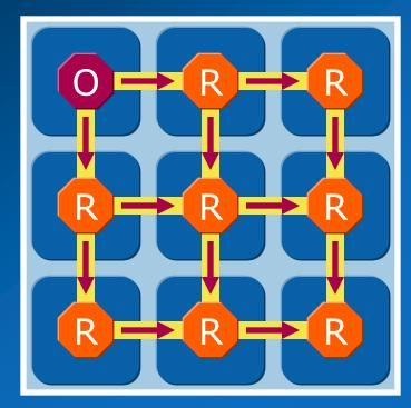
*Assume: 10mm die, 1.5u bus pitch 50ps repeater delay*  **Arbitration:** Each cycle for the next cycle Decision visible to all nodes
