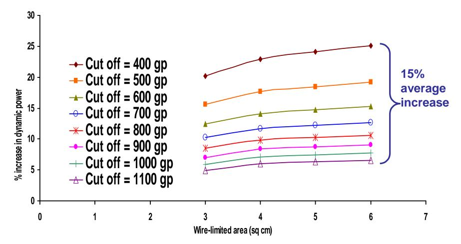
Interconnect elimination does not result in any power reduction
